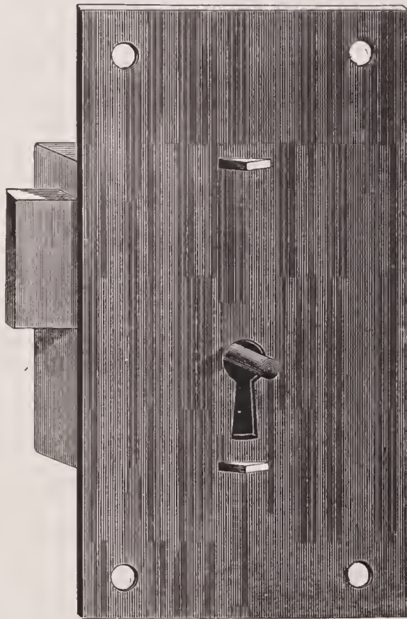
No. 714. 4 x 2 1/4 inch, $2.50. Iron. Solid Square Box, Broad Heavy Bolt, shoots right and left, 2 Secure Levers, Fancy Bow Keys, all different.
